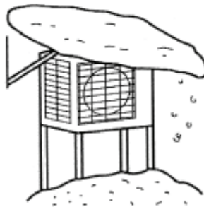
Figure 1: construction of canopy and pedestal
