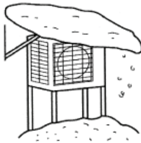
Figure 1: construction of canopy and pedestal
